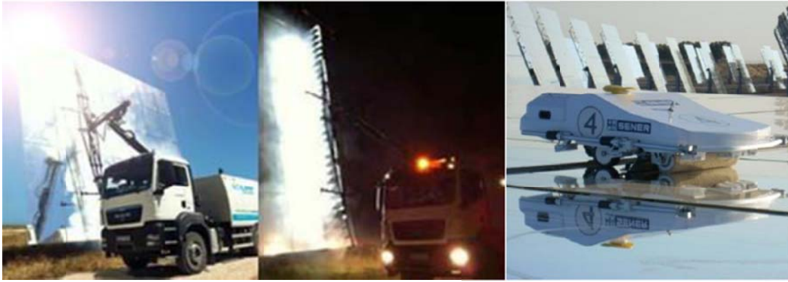
Fig. 2. Heliostat cleaning: Pressurized water jet cleaning with a truck (left, centre); and mechanical cleaning (sweeping/wiping) with the robot-based HECTOR system (right). Images from Burgaleta et al. (2012).
